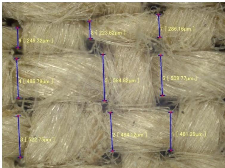
**Fig. 2-5 Measurement of the width of the force-bearing hemp**
