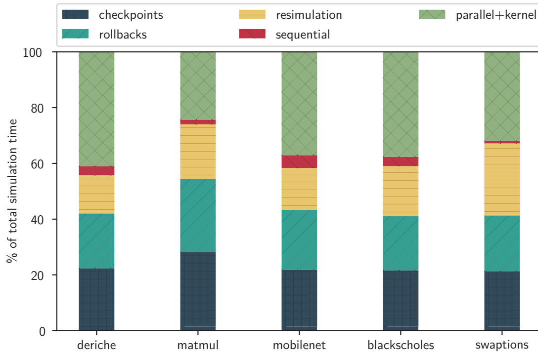
Figure 5.1 – Analysis of the time spent in parallel and sequential simulation, in checkpointing and rollback procedures as well as the overhead caused by re-simulation after rollback, when using 8 workers (the trend is the same with all numbers of workers). It should be noted that non-parallel simulated code can still be simulated during the parallel phase. Thus, the sequential time only reflects the amount of time spent in sequential evaluation phases, not the nature of the simulated code.
