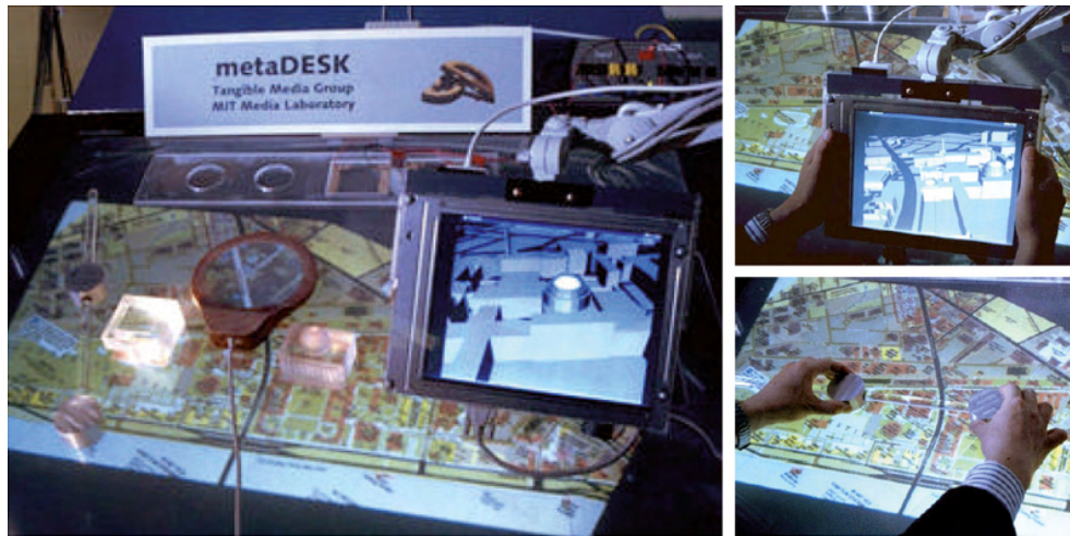
Figure 2.7: (Left) The metaDESK with tangible elements: lenses, phicons, and instrument [191]. (Right top) Demonstration of the activeLENS. The device provides a bird's-eye view of a place where it is over the map. (Right bottom) The instrument can scale and rotate the map. Courtesy of Tangible Media Group, MIT Media Lab.
