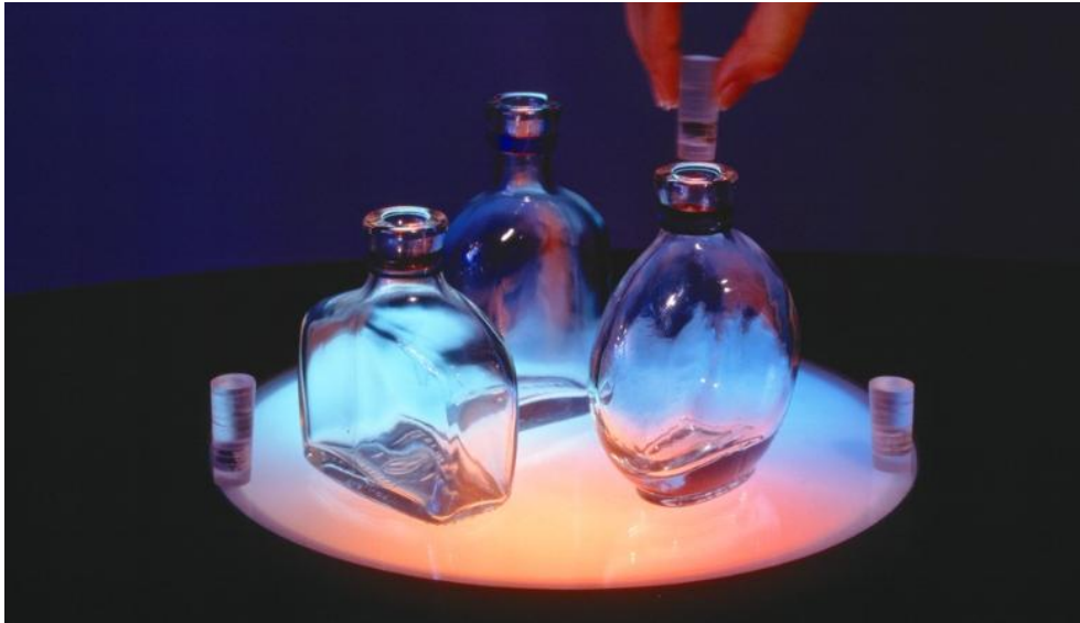
Figure 2.5: MusicBottles, a PUI for playing jazz music. Users can control which instrument of the music is played by opening and closing the bottle lids [83]. Courtesy of Tangible Media Group, MIT Media Lab [175].
