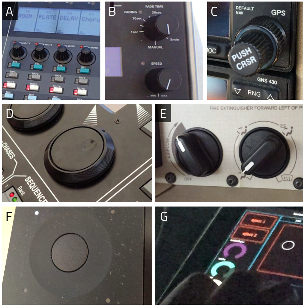
Figure 3.13: Examples of rotational controls we observed in the contextual interviews. (A) Continuous dials with infinite ranges. (B) Dials with discrete visual markers. (C) Two-leveled dials with detents, enabling both coarse and precise controls depending on which level users are controlling. (D) a shuttle dial with a smooth concave notch. (E) an arrow-shaped dial with a limited control range. (F) a tactile dial on a graphic tablet. The round groove allows users to place and move fingers on it. (G) tactile dials on a touchscreen tablet. They control continuous and bounded parameters.
