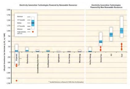
**Fig. 1.7** Estimates of lifecycle GHG emissions of electricity generation technologies.
