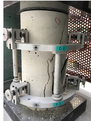
(b) Essai de compression
