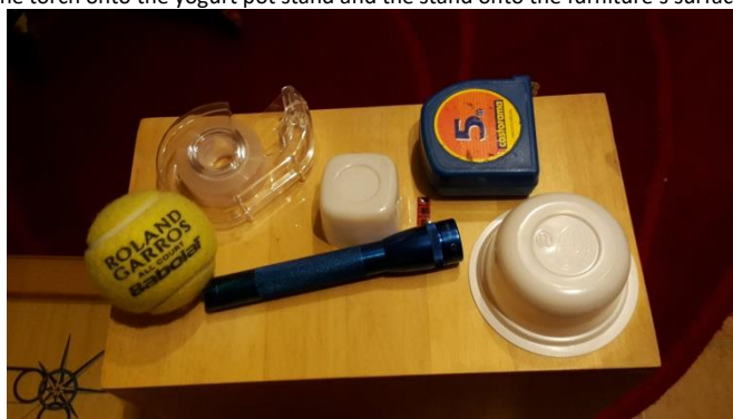
Figure 1: picture of the main items needed for the shadow method to measure the diameter d of a tennis ball.
