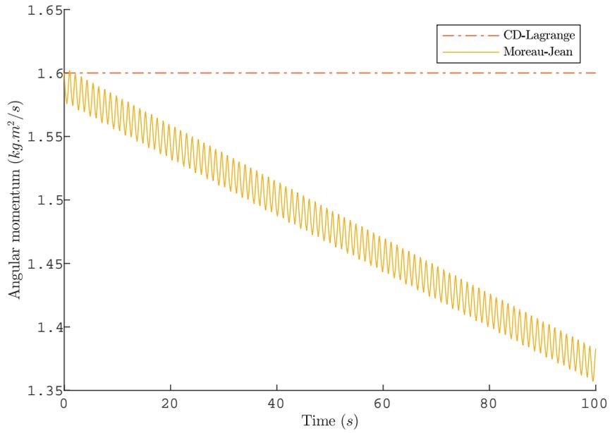
Figure 2.12: Rotating spring – Angular momentum
