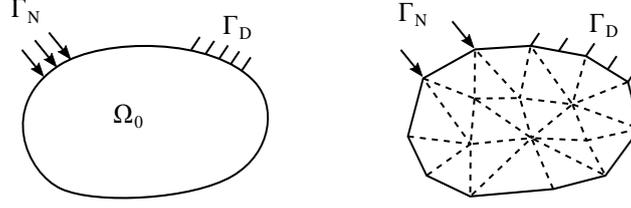
Figure 1.2: Spatial discretization of a deformable body
