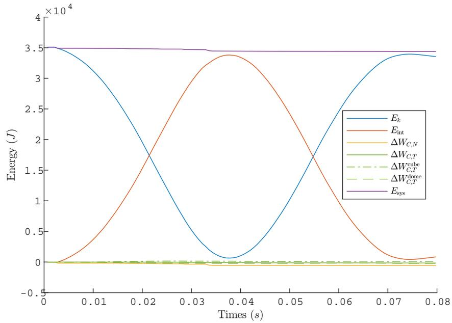
Figure 4.22: Energy balance on mesh 3 – Friction with sticking contact
