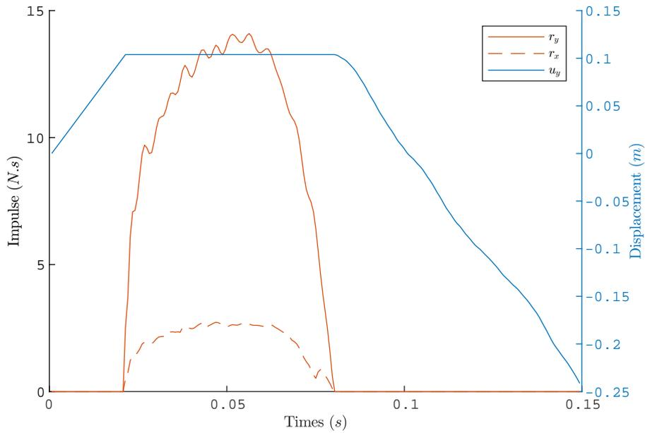
Figure 2.20: Impacting dome – Impulses and contact displacement
