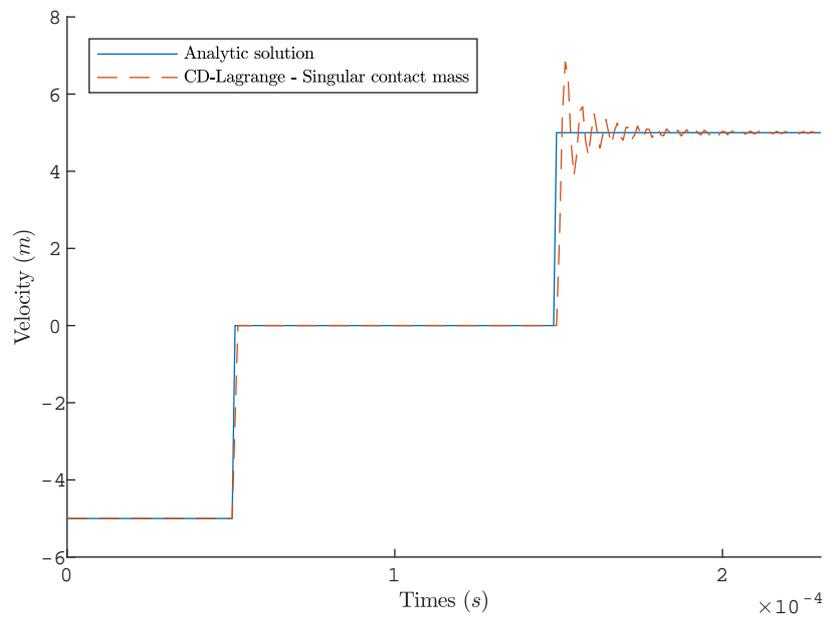
Figure 3.3: Singular impacting bar – Velocity of contact node
