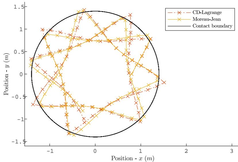
Figure 2.11: Rotating spring – Position over 10 s
