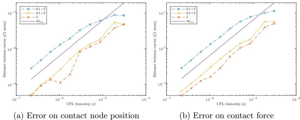
Figure 3.9: Singular impacting bar – Convergence rates
