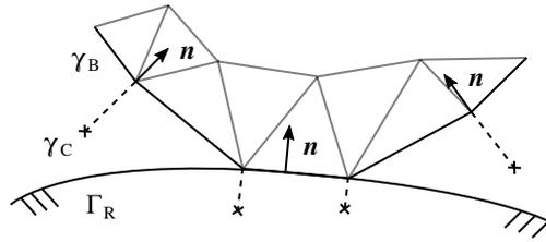
Figure 3.10: 3D formulation – Normal massless elements
