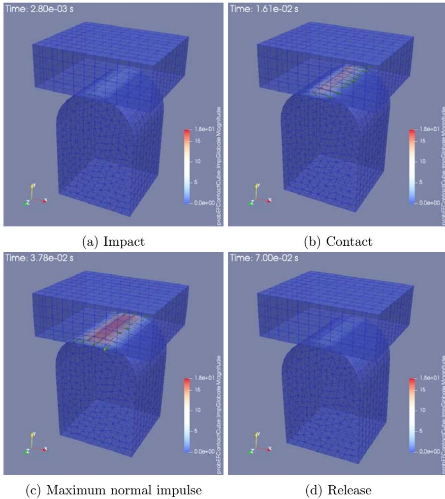
Figure 4.21: Deformation of mesh 3 – Friction and sticking contact
