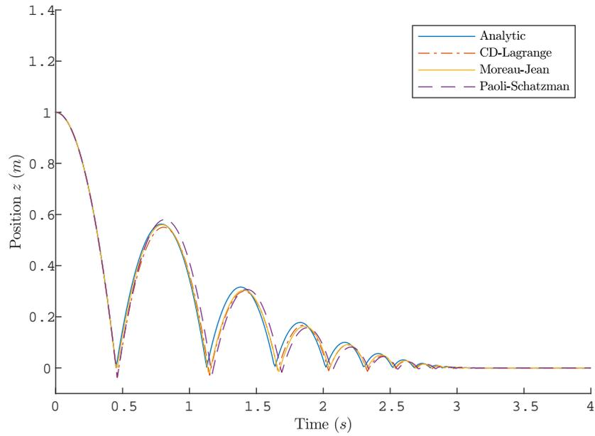
Figure 2.3: Bouncing ball – Position for  $e_c = 0.75$
