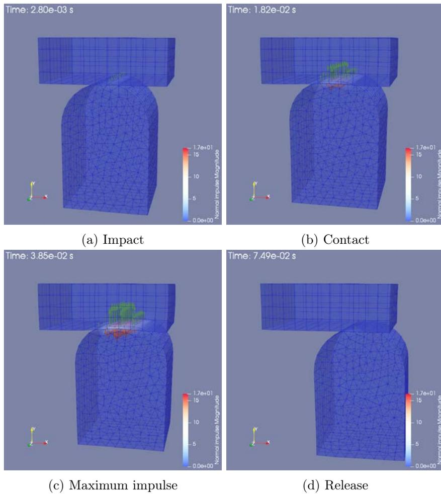
Figure 4.15: Deformation on mesh 3 – No-friction and large sliding
