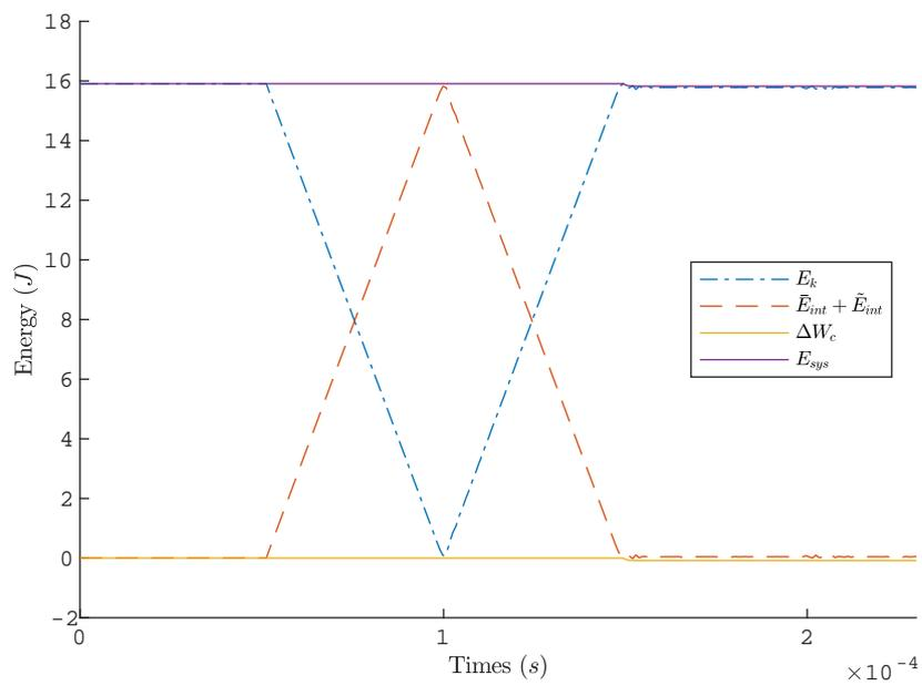
Figure 3.5: Singular impacting bar – Energy balance
