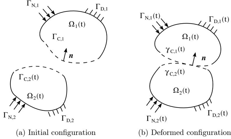
Figure 4.1: Contact between two deformable bodies
