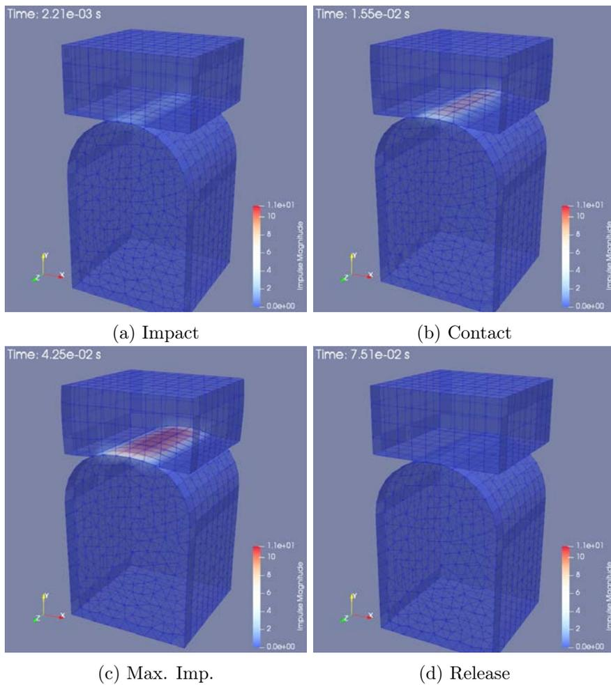
Figure 4.9: Deformation on mesh 3 – Lumped mortar
