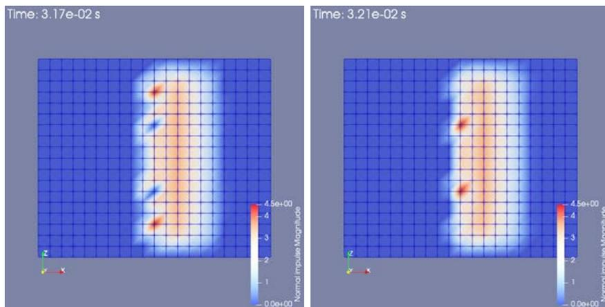
Figure 4.19: Cube contact side for mesh 5 – No-friction and large sliding
