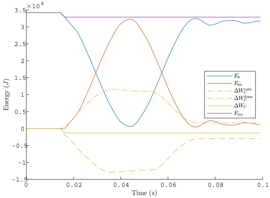
Figure 4.7: Energy balance on mesh 1 – Non-lumped mortar
