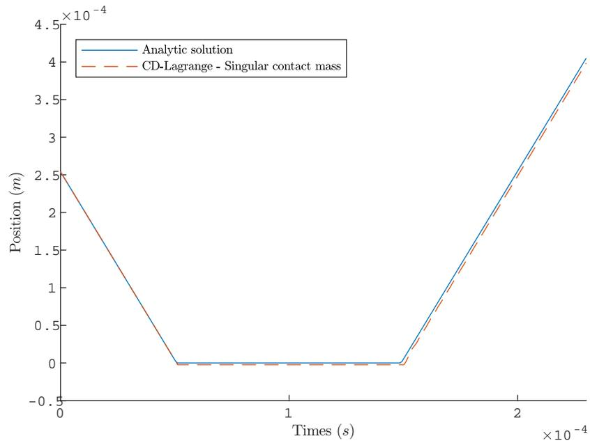
Figure 3.2: Singular impacting bar – Position of contact node
