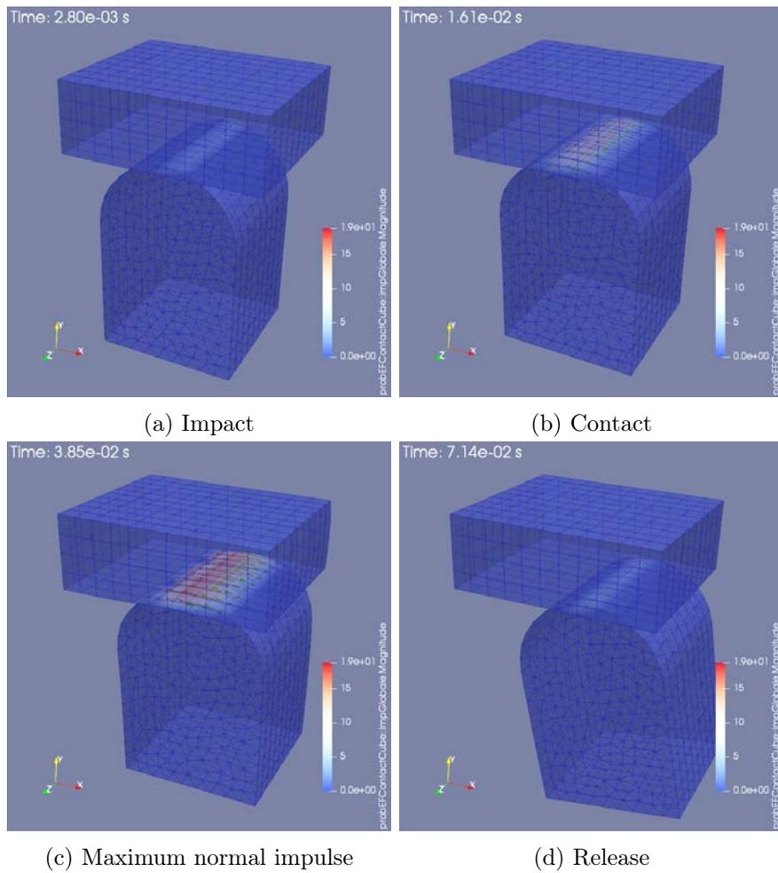
Figure 4.25: Deformation on mesh 3 – Friction and sliding contact
