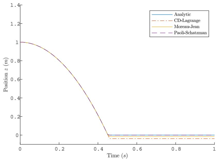
Figure 2.4: Bouncing ball – Position for  $e_c = 0$
