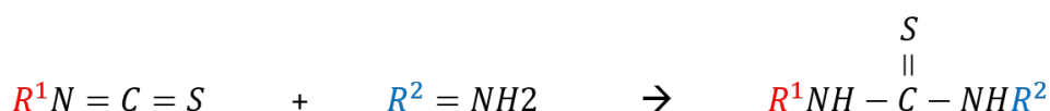
Figure 4.2: Chemical acylation reaction between an isothiocyanate group and a primary amino group
