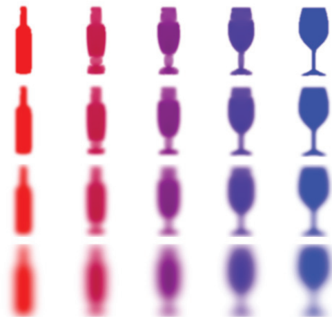
Figure 2.6: Influence of the entropic regularization for barycenters in dimension 2. Barycentric interpolation between 2 distributions (on each row), for different values of \epsilon , top to bottom 3 \cdot 10^{-4} , 1 \cdot 10^{-3} , 3 \cdot 10^{-3} , 1 \cdot 10^{-2} , and L = 200 iterations.
