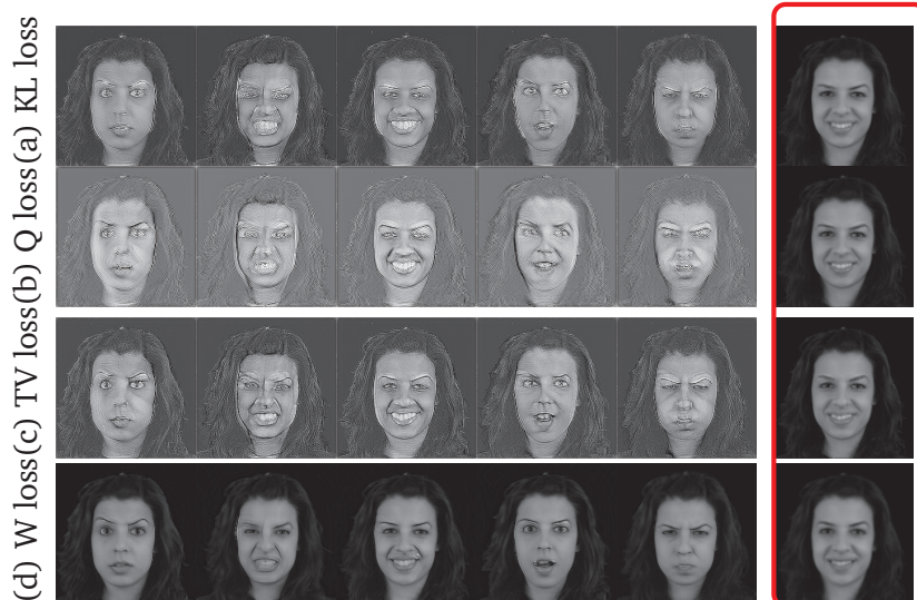
Figure 3.7: Similarly to Figure 3.6 , we compare the atoms obtained using different loss functions, ranking them by mean PSNR: (a) \overline{PSNR} = 33.81 , (b) \overline{PSNR} = 33.72 , (c) \overline{PSNR} = 32.95 and (d) \overline{PSNR} = 32.34
