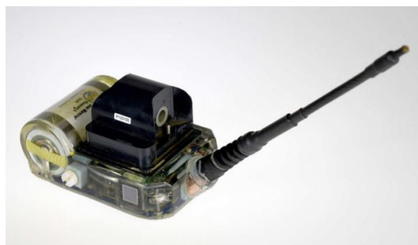
Figure 17 : Balise Conductivity-Temperature-Depth Satellite-Relayed Data Loggers (CTD-SRDL).
