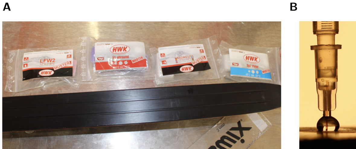
Figure 5.10: (A) Ski sole with the different tested waxes. (B) Contact angle measurement.
