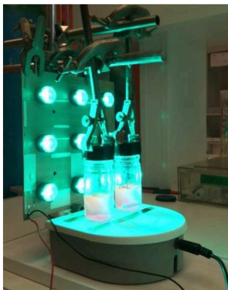
Figure III.10: Homebuilt photocatalysis setup using cyan light ( \lambda = 501 \text{ nm} ) produced by nine LEDs. The irradiated vials contain suspensions of \text{Gd}_{2(1-x)}\text{Ce}_{2x}\text{O}_2\text{S} nanoparticles in aqueous rhodamine B solutions. During the reaction, the setup was kept in the dark.
