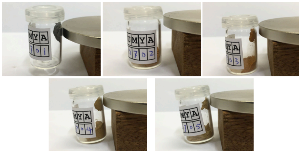
Fig 78. Magnet test of an iron powder sample before the reaction (01), and after the reaction: batch 1 (02), batch 2 (03), batch 3 (04) and batch 4 (05).
