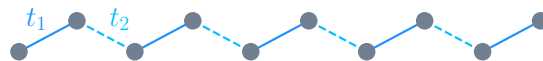
Figure 2.5 An SSH chain of 10 sites. The unit cell is made of two neighboring sites, with hopping t_1 ( t_2 ) between sites belonging to the same (different) unit cell.
