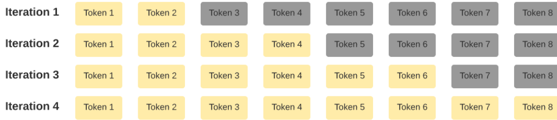
Figure 4.4: Example of how the decoder is fed by chunks of text progressively
