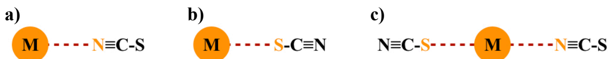
Schéma 6. a) mode N-terminal (ligand isothiocyanato) ; b) mode S-terminal (ligand thiocyanato) ; c) mode pontant.
