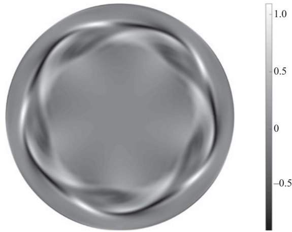
FIGURE 19. Axial vorticity of the fluctuations at the interface, DNS with frozen condition u_r = 0 at the interface for Re = 18\,620 .
