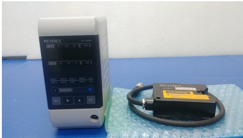
Figure VII.1 – LK-GD500 controller (left), with Keyence LK-G10 sensor (right) .
