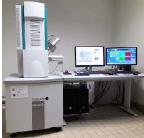
Figure 2.16: Instrument EMB-EDX (Microscopie Electronique à Balayage) used for EDX measurements.
