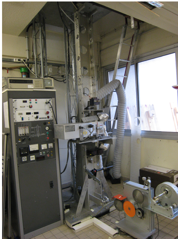
Figure 1.41: (a) The essential components of a drawing tower, are a preform feed mechanism, a furnace, a diameter monitor, a resin-coating applicator, a UV furnace, a guide pulley, an attraction capstan, and a take-up unit. (b) Picture of the drawing tower used at INPHYNI.
