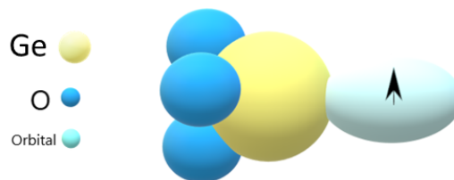
Figure 1.26: Microscopic structure of GeE' center.
