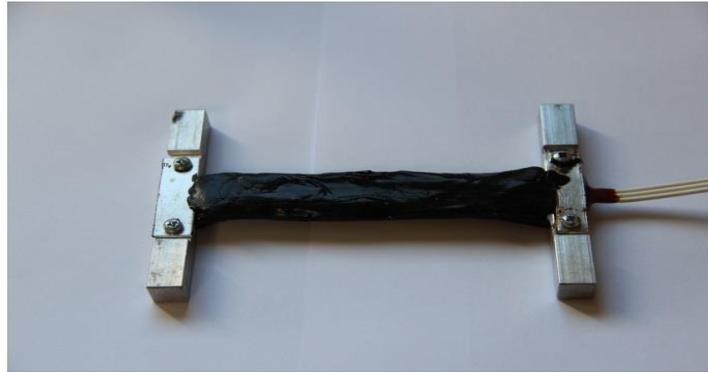
Figure 1-25. KM-120-120-H211W1M3 type strain gauge
