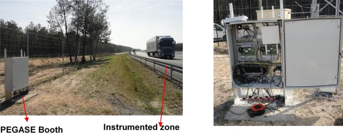
Figure 5-4 (a): Instrumented site (Duong et al., 2020) (b): Road side box with the peagse boards and transmitters
