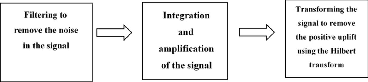
Figure 3-9. Signal Treatment method
