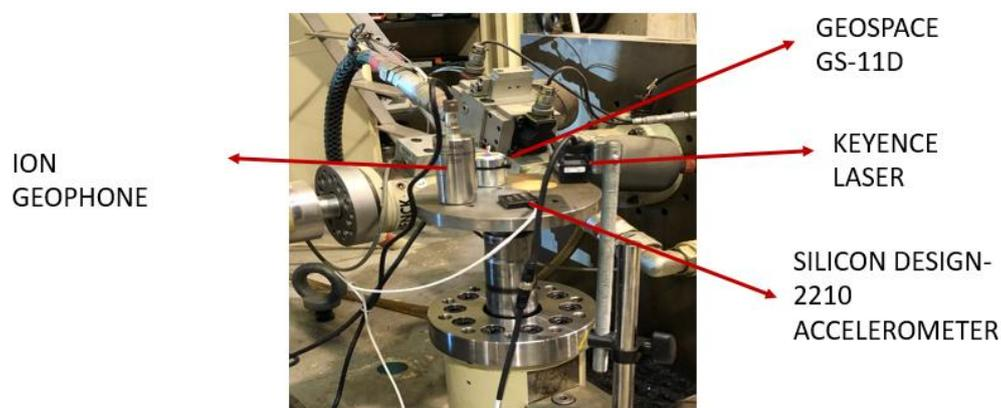
Figure 2-4. Vibrating table with various sensors attached to test
