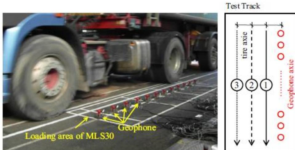
Figure 1-34. Geophone experimental setup on the test section and test vehicle (Liu et al., 2017)
