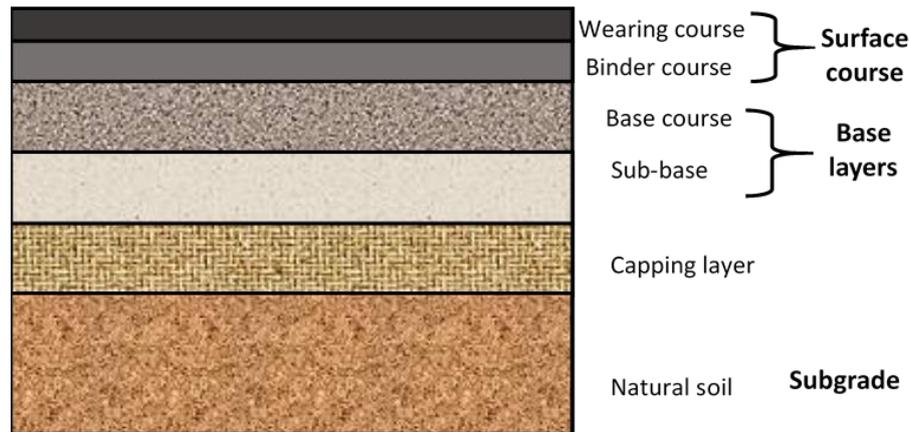
Figure 1-1. Composition of a pavement structure
