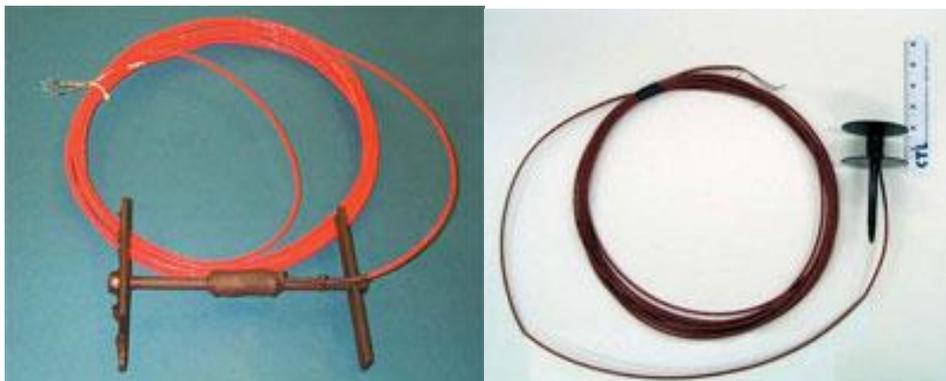
Figure 1-28. Horizontal and vertical CTL gauges
