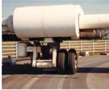
Figure 3-2. Loading configurations used for the test: dual wheel
