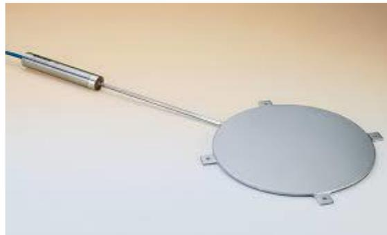
Figure 1-30. Hydraulic pressure cell
