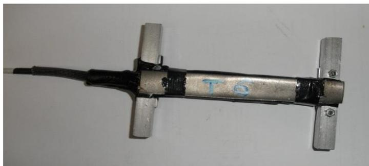
Figure 1-26. Aluminum support strain gauge
