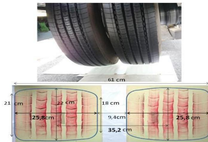
Figure 3-3. Dual wheel load dimensions
