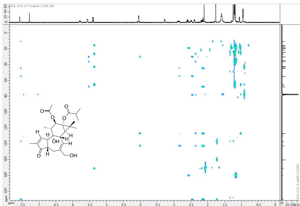
Figure S49. HMBC spectrum of 4-dPE B (**18**) (500 MHz, CDCl<sub>3</sub>, 300 K)
