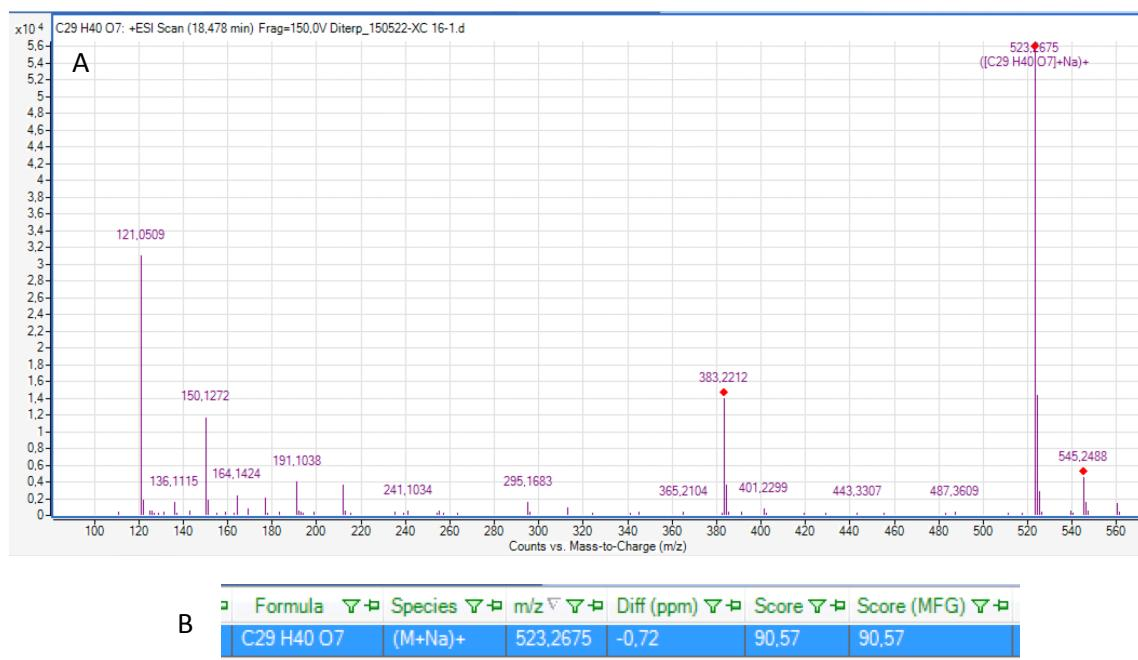
Figure S28. ESI-HRMS/MS of  $4\alpha$ -dPE A (**16**) (Q-TOF). (A) ESI-HRMS/MS spectra of  $m/z$  523.2675. (B) Zoom on backbone ions
