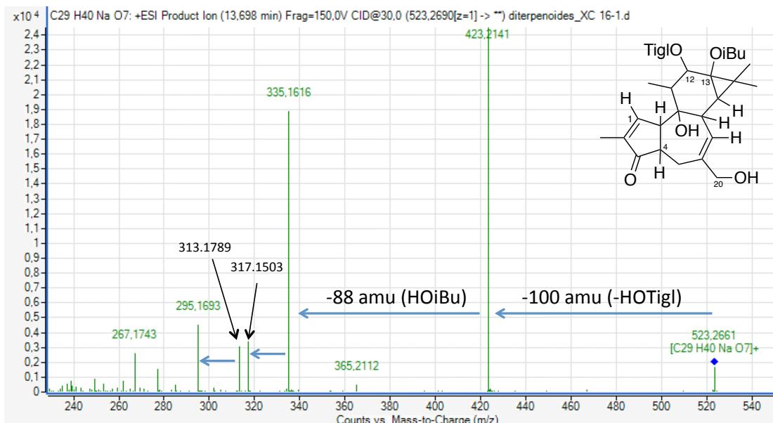
Figure 3. ESI-HRMS/MS spectrum of  $m/z$  523.2661 at 13.7 min was annotated as 4-deoxyphorbol 12-tiglyloxy-13-isobutyrate based on its previous isolation in this species.<sup>5</sup> (HOTigl = tigloic acid ; HOiBu = isobutyric acid).
