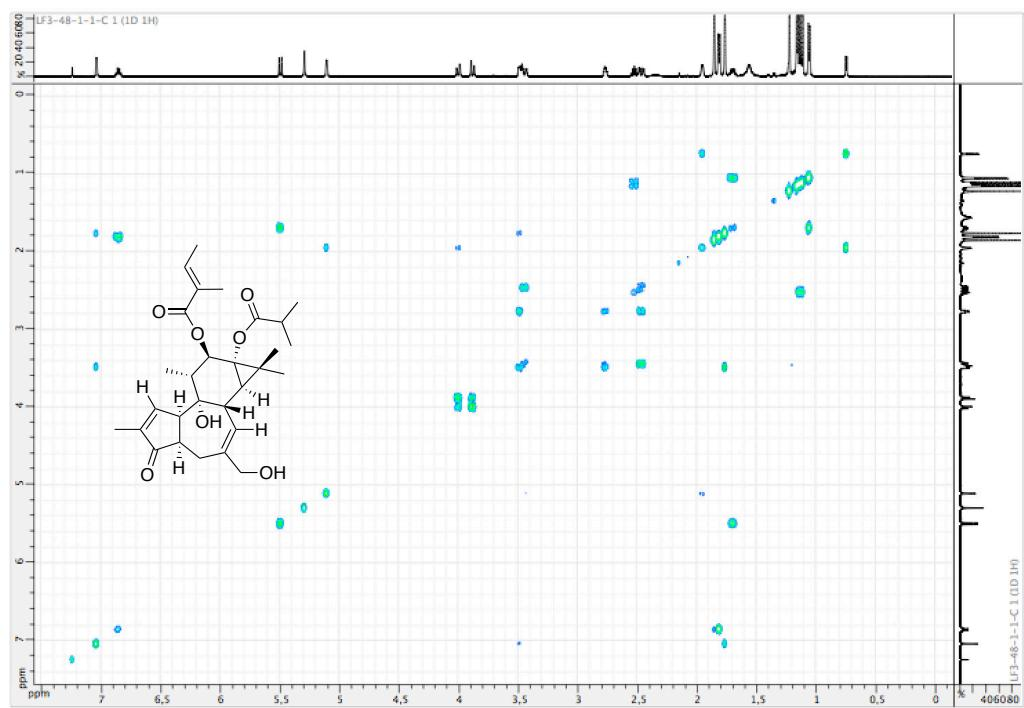
Figure S32. HSQC spectrum of  $4\alpha$ -dPE A (**16**) (500 MHz,  $\text{CDCl}_3$ , 300 K)
