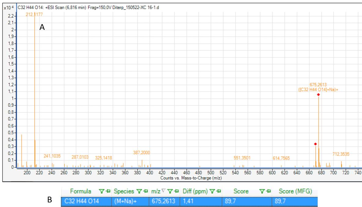
Figure S2. ESI-HRMS/MS of JE-C1 (**13**) (Q-TOF). (A) ESI-HRMS/MS spectra of  $m/z$  675.2611. (B) Zoom on diterpene backbone ions
