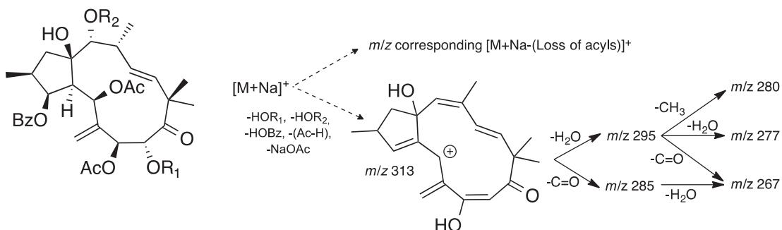
**Fig. 11.** ESI-MS<sup>2</sup> fragmentation behavior of JE from group A (11–17) and group B (18–22) in ESI positive ion mode observed using hybrid QqQ/linear ion trap and hybrid linear ion trap/Orbitrap mass spectrometers.
