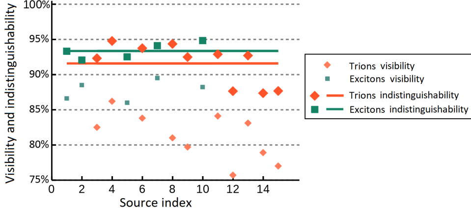
Figure 2.22: Measured visibility V of the photons (smaller points) and single-photon indistinguishability M_s , measured when the sources were tuned for maximum brightness. The green squares represent sources based on excitons; the orange diamonds sources based on trions. The horizontal solid lines show the mean value of indistinguishability for each type of source.
