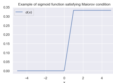
Figure 6.2: Sigmoid function satisfying the Maiorov condition with \varphi(x) = \frac{x+1}{3} \mathbb{1}_{[-1,0]}(x) + \frac{1-x}{3} \mathbb{1}_{[0,1]}(x)
