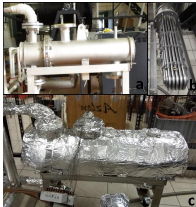
Figure 6. 2 Modified LHTES system. a) outer shell without insulation b) tubes inside the shell c) insulated system
