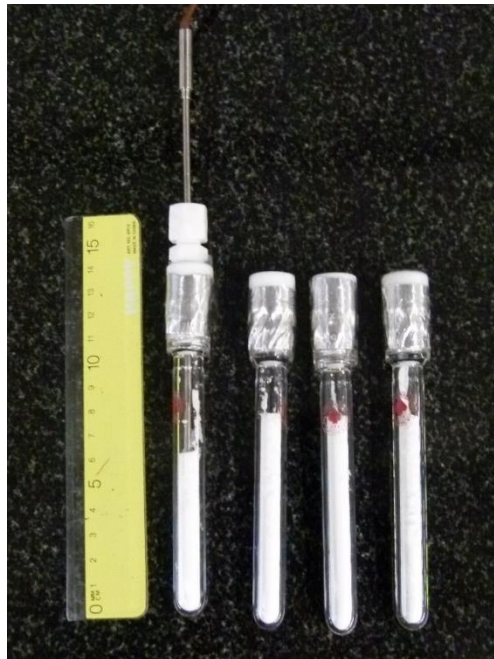
Figure 4. 6 U-SN eutectic samples for thermal cycling tests
