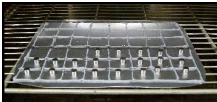
Figure 3. 2 The sample rack with some of the samples in it inside the heating cabinet
