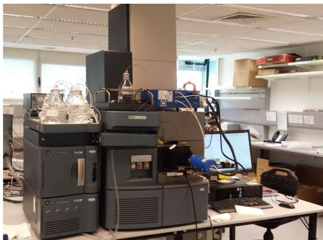
Figure II-19 : Instrument DART-TOF-MS
