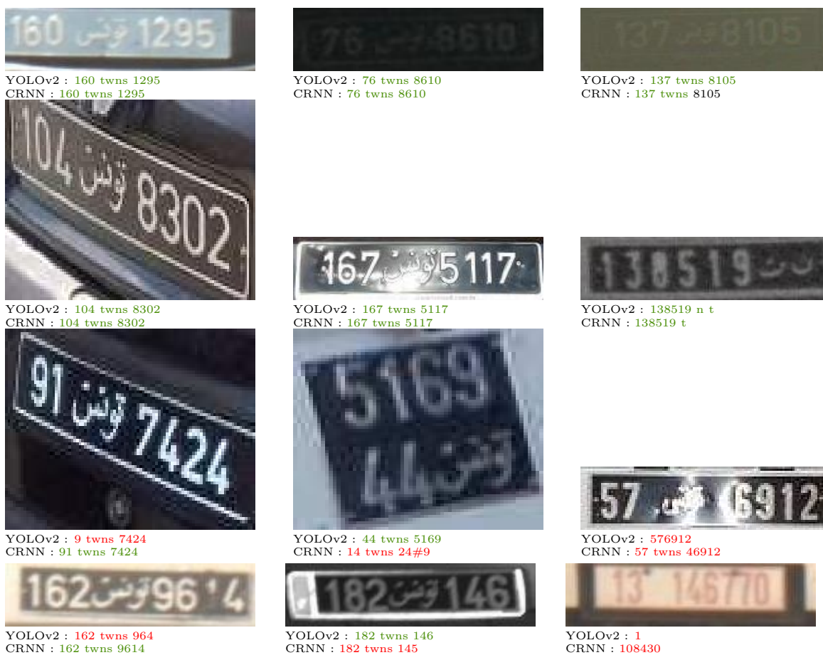
Figure 3.10: Qualitative results obtained by the proposed ALPR system in the GAP-LP and Radar datasets. Green text refers to correctly recognized LP, while miss-recognized LP are written in red.
