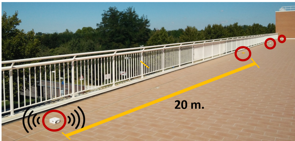
Fig. 6.5: The deployment of one line of sensors
