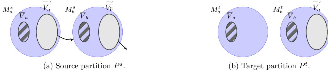
Figure 5.4 – Illustrative example for Property 5.2.a, where vertices in \vec{V}_a (resp. \vec{V}_b ) move from their source module M_a^s (resp. M_b^s ) (Fig. 5.4.a) into target module M_b^t (resp. M_c^t , which is purposely not shown) (Fig. 5.4.b). \vec{V}_a and \vec{V}_b represent the non-moving vertices.
