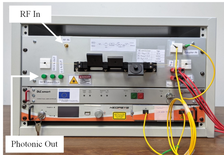
Figure E.2 Rack box used to arrange the components required for photonic generation and modulation of the optical tones (except for the mm-wave photonic Tx and OSA).
