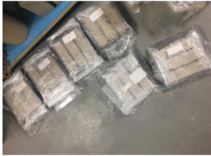
Figure 2.57: Storage of the samples before demoulding
