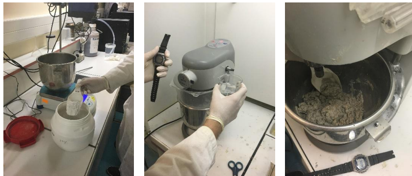
Figure 2.55: Procedure of the mortar preparation
