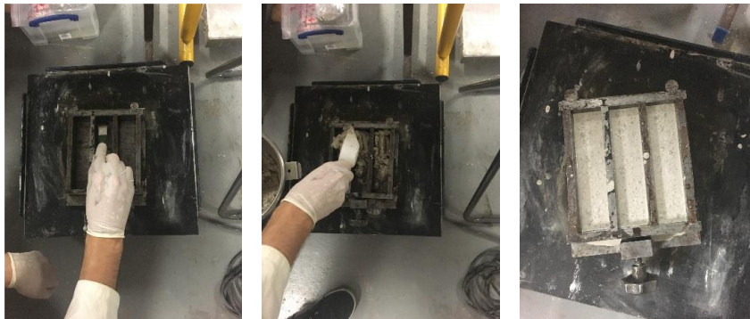
Figure 2.56: Filling procedure of the prismatic moulds
