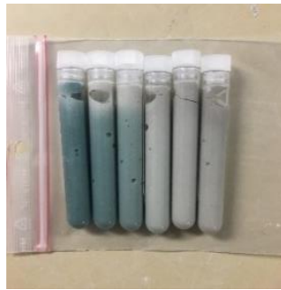
Figure 2.70: Paste samples for ex-situ Laboratory XRD analysis
