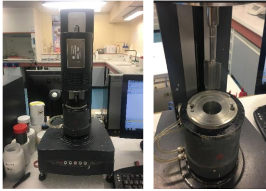
Figure 2.23: Rheometer from TA Instrument with vane-in-cylinder geometry used in this study
