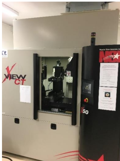
Figure 3.36: X-ray CT scanner for non-destructive microtomography observation of the sample 3D microstructure
