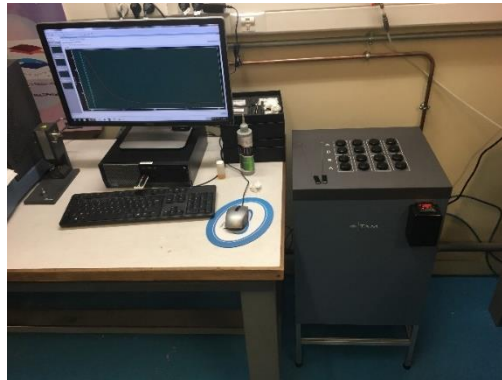
Figure 2.36: TAM Air Isothermal micro-calorimetry equipment for heat evolution recording during the binder paste hydration process
