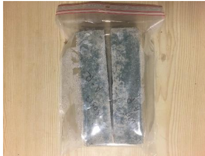
Figure 2.58: Further storage of the samples in plastic bags after demoulding
