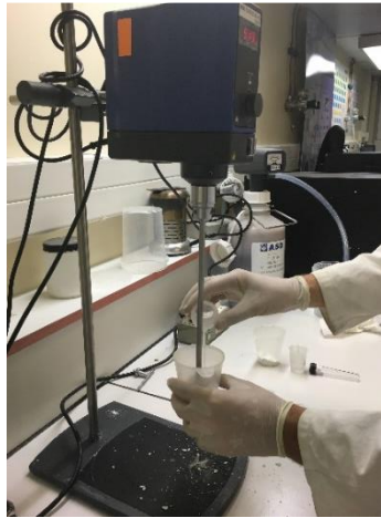
Figure 2.24: Preparation of paste sample
