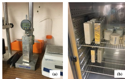
Figure 4.26: Procedure for measurements of longitudinal dimensional variation of the mortar samples (a) and sample storage in climatic chamber (b)
