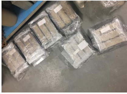
Figure 2.57: Storage of the samples before demoulding
