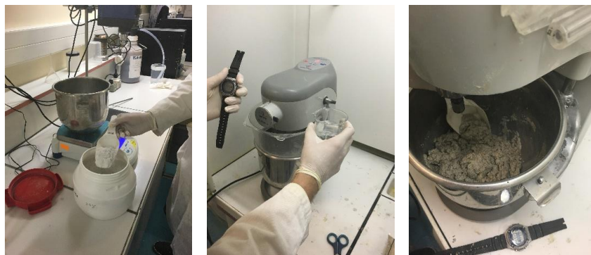
Figure 2.55: Procedure of the mortar preparation
