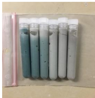
Figure 2.70: Paste samples for ex-situ Laboratory XRD analysis
