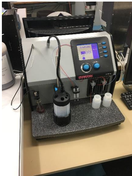
Figure 2.15: ZetaProbe Analyser for measurement of particle surface charge
