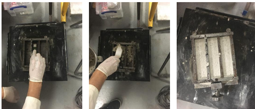
Figure 2.56: Filling procedure of the prismatic moulds
