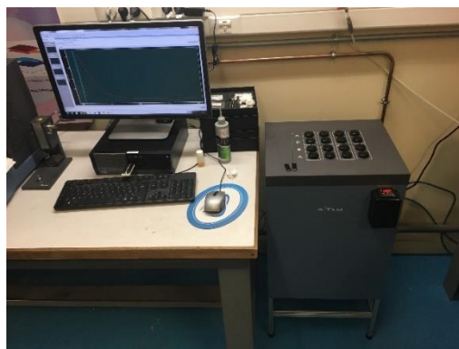
Figure 2.36: TAM Air Isothermal micro-calorimetry equipment for heat evolution recording during the binder paste hydration process
