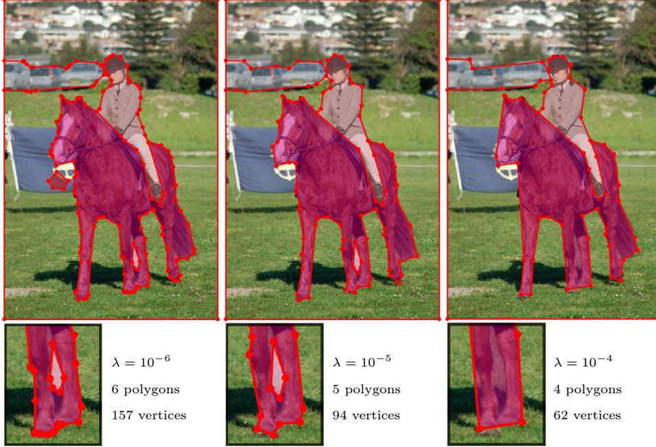
Figure 3.2: Trade-off between fidelity to data and complexity to output polygons. Increasing  $\lambda$  gives more compact, yet less accurate, output polygons. Objects of interest: horses, persons and cars.
