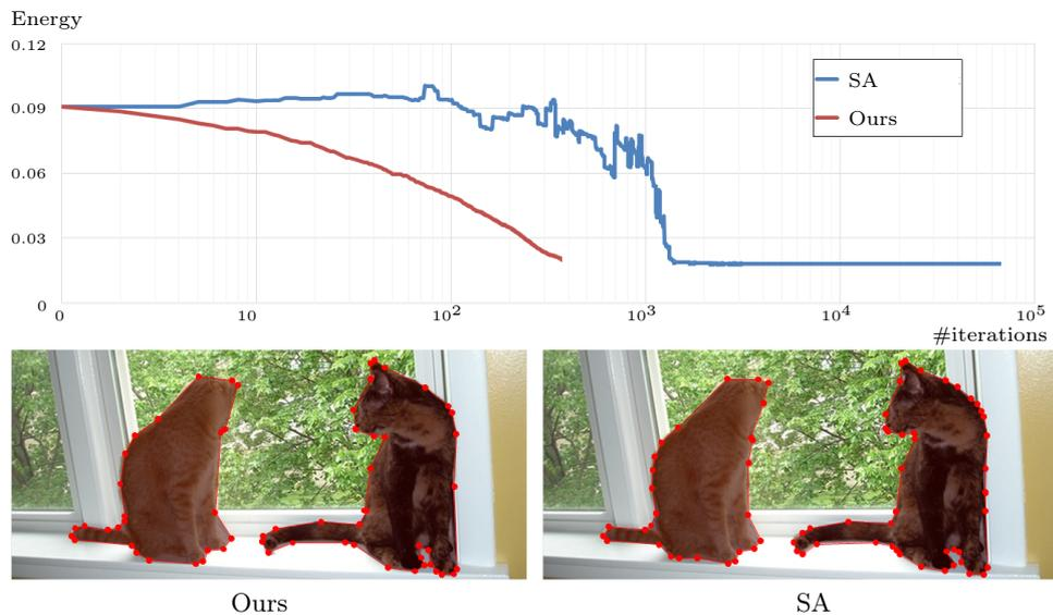
Figure 3.6: Evolution of energy  $U$  during our exploration mechanism (red curve) and a simulated annealing optimization (SA, blue curve). While the two optimization techniques converge towards a similar energy, our exploration mechanism requires two orders of magnitude less iterations than the simulated annealing.
