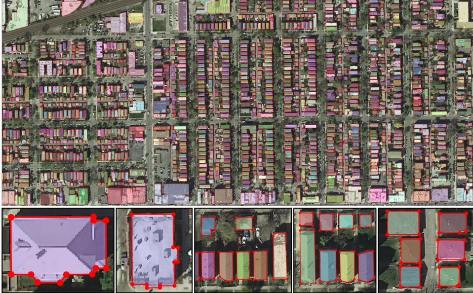
Figure 3.10: Extraction of buildings from satellite images with our algorithm: 1,178 buildings of a half square kilometer area of Chicago, USA, are extracted with low complexity polygons (8,683 vertices). While compact, the polygons capture some fine details (see closeups).
