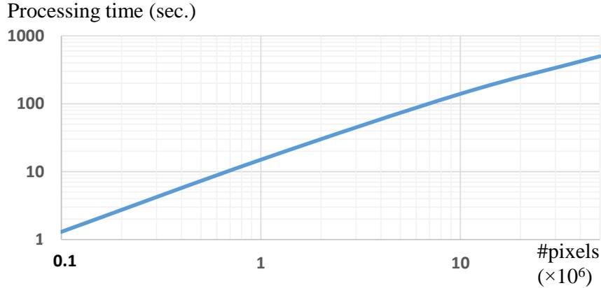
Figure 3.11: Processing time against number of pixels in the input image.
