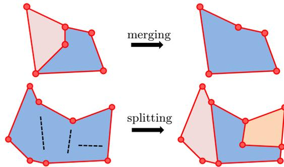
Figure 3.5: Merging and splitting operators. The merging operator merges two adjacent facets with different semantic labels by removing the common edges (top). The splitting operator divides one facet into multiple facets that have different semantic labels (bottom). The black dashed lines indicates the cutting directions detected in the input image (bottom left).
