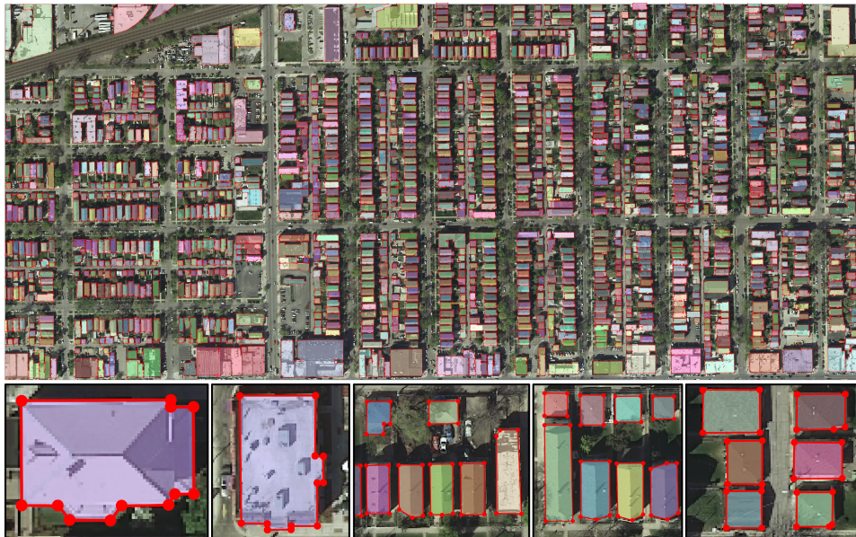
Figure 3.10: Extraction of buildings from satellite images with our algorithm: 1,178 buildings of a half square kilometer area of Chicago, USA, are extracted with low complexity polygons (8,683 vertices). While compact, the polygons capture some fine details (see closeups).
