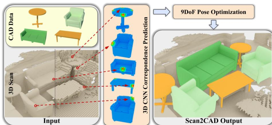
Figure 2.9: An example of CAD model alignment against input depth scans via a 3D CNN approach, which predicts heatmap correspondences between the scan and the CAD model. Image taken from [ADD<sup>+</sup>19].
