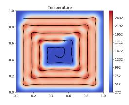
Figure 2.9: Interior spiral path at time t=0.87.
