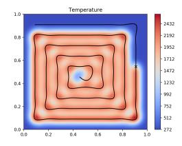
Figure 2.10: Exterior spiral path at time t=0.87.
