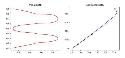
Figure 2.13: Initial and optimized path
