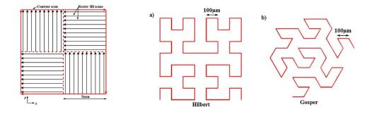
Figure 2.5: Illustration of island scan control sample and scan strategies generated using (a) Hilbert and (b) Peano-Gosper mathematical space filling curves as studied in [11].
