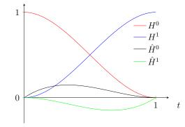
Figure 2.7: Hermite basis functions.
