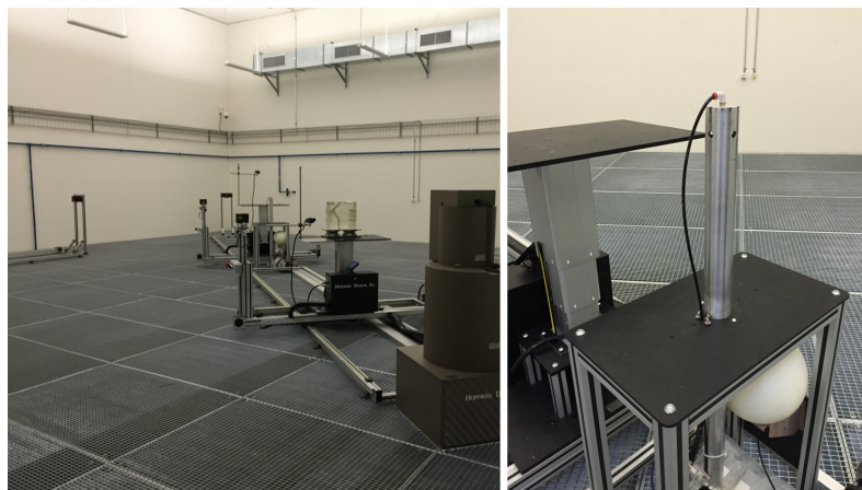
Figure 5.7: Am-Be irradiation room to the left and source exposure position to the right.
