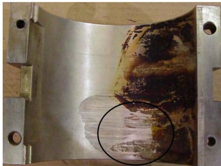
**Figure 1.7.** An example of babbitt material creep in a cylindrical bearing [46].
