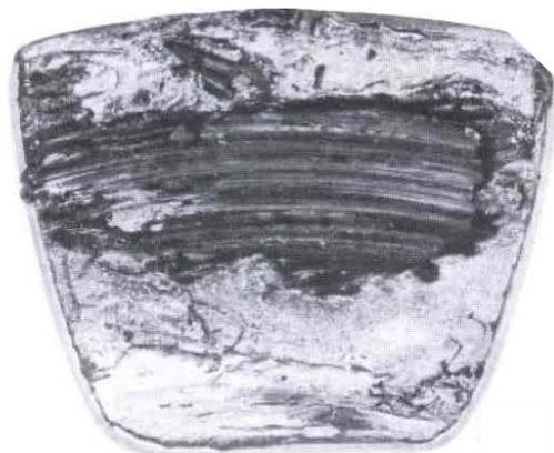
**(b)** Wire wooling on a thrust pad.
