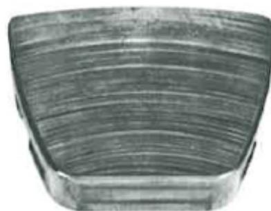
**(b)** Concentric scoring of a thrust pad.
