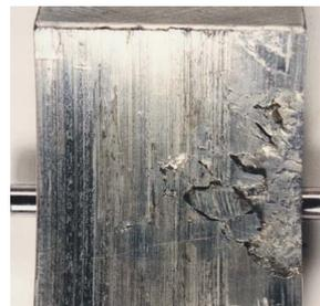
(b) Babbitt mechanical fatigue on a tilting pad.
