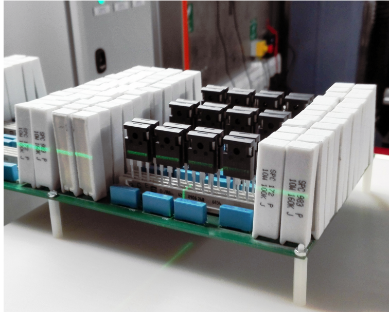
Figure 3.4: Photo of the test board with SiC MOSFETs placed in neutron irradiation test position.
