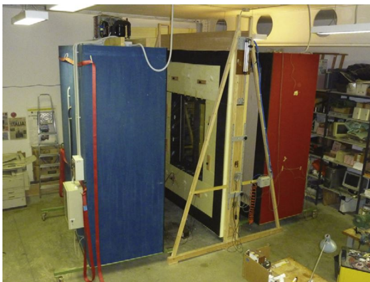
Figure 2.6.: General view of the hot box apparatus from Asdrubali and Baldinelli [59].
