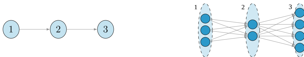
Figure 2.2 – A sequence of customers in the auxiliary network for the ATSP and its generalization to delivery options in the GVRPTW
