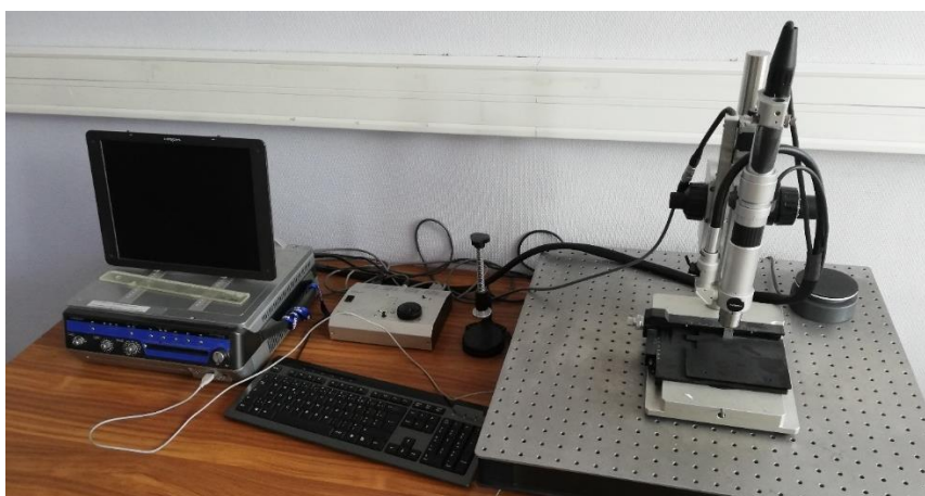
Fig. A - 6 Digital Optical Microscopy Hirox in Laboratoire de Mateis in INSA de Lyon, France
