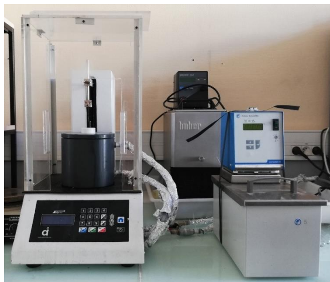
Fig. II.4 - 1 Dip-coating machine connected with heat container and heat generator
