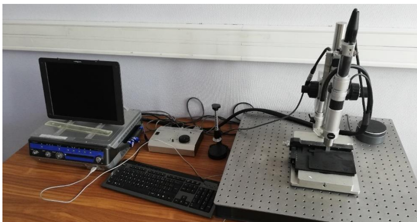
Fig. A - 6 Digital Optical Microscopy Hirox in Laboratoire de Mateis in INSA de Lyon, France
