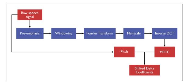
Figure 2.13: Pipeline for MFCC-SDC feature extraction.
