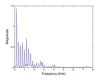
Figure 2.16: Magnitude of the frequency spectrum obtained with a DFT of the pre-emphasized and windowed segment of the vowel [v] shown before.
