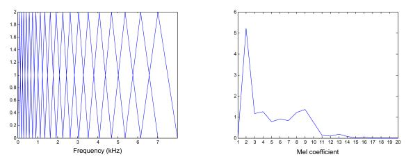
Figure 2.17: Triangular Mel filters (left), and magnitude of the Mel-frequency spectrum (right) after applying the filter bank to the DFT spectrum shown before.
