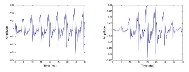
Figure 2.15: A 40 ms frame of the vowel [v] segmented from a Catalan utterance, before (left) and after (right) applying a *Hamming window* function.
