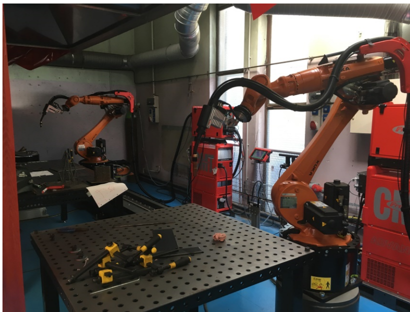
Figure 2.2 – Plateforme Pro3D WAAM (IUT de Nîmes).
