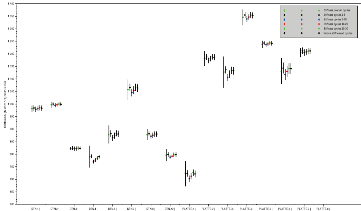
Figure 62: Mean±2SD compressive stiffness construct values for all samples over all cycles, cycles 2-5, cycles 5-10, cycles 10-20, cycles 20-30, and the robust stiffness calculation (over all cycles) during phase 2 of testing at 350 N (stiffness calculated at 200±100 N).
