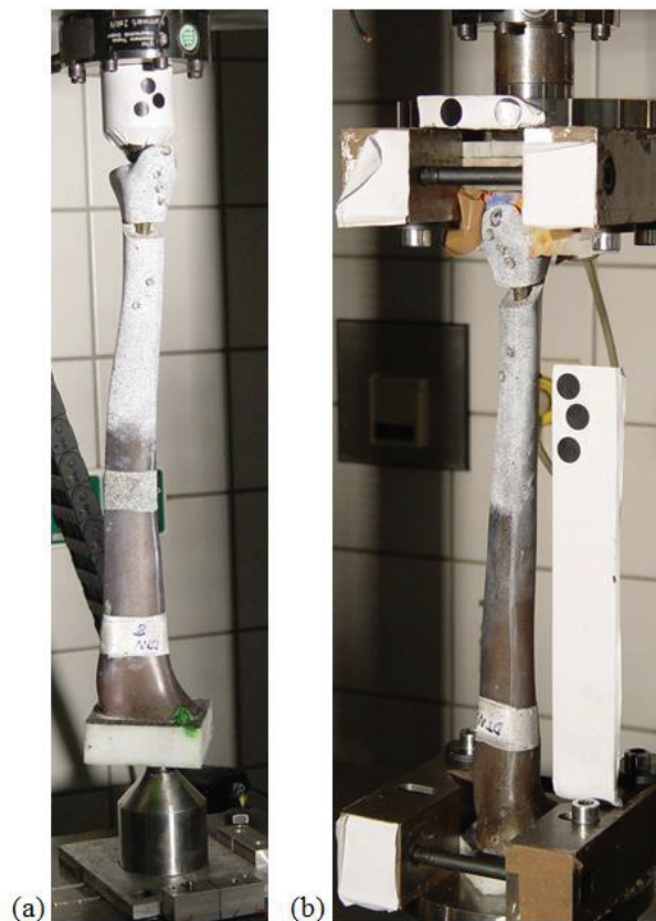
Figure 35: Marker placing on the machine clamps for tracking during compression (a) and torsional (b) testing.
