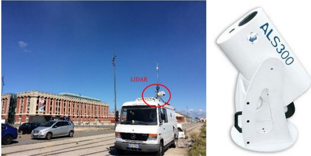
Figure III-2 LIDAR system installed in an atmospheric mobile unit.
