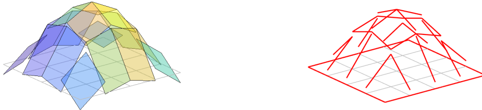
Figure 1.5 Representation of the HHO DoFs as broken polynomials of degree k = 1 on the mesh (left) and its skeleton (right)
