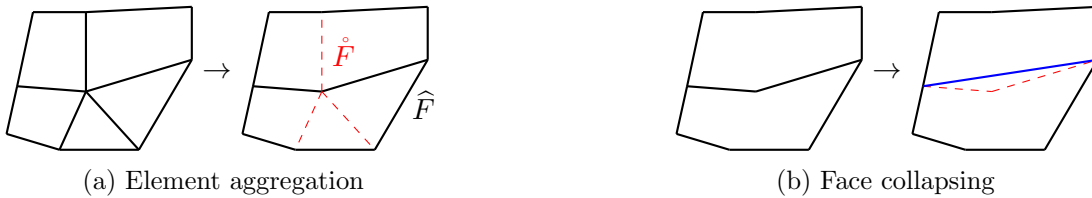
Figure 5.2 Aggregation process with face collapsing. In (a), elements are aggregated, yielding two aggregates. “Removed” edges, represented in dashed red lines, are collected in \mathring{F} , while the remaining ones are collected in \hat{F} . Then, in (b), the interface between the two neighbouring aggregates, here made of two edges (in dashed red lines), is collapsed into a single one (solid blue line). The other edges yield singleton face aggregates.
