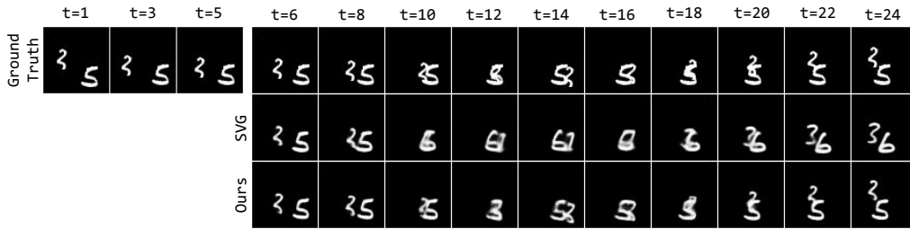
Figure 5.3 – Conditioning frames and corresponding ground truth and best samples with respect to PSNR from SVG and our method for an example of the SM-MNIST dataset.
