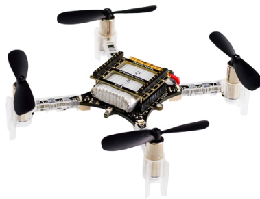
FIGURE E.11: Photographie du Crazyflie 2.0 (source: www.bitcraze.io/products/old-products/crazyflie-2-0/ )
