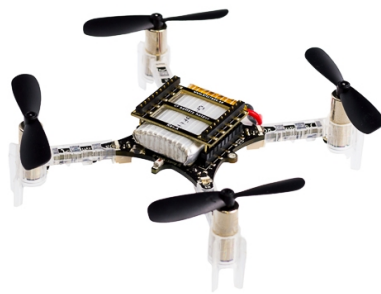
FIGURE 4.8: Picture of the Crazyflie 2.0 (source: www.bitcraze.io/products/old-products/crazyflie-2-0/ )
