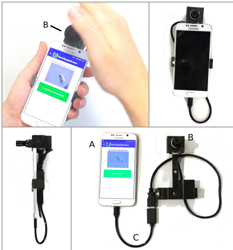
Figure 20: A neuromorphic camera (an ATIS) (B) is plugged into a smartphone (A) using a USB link (C), allowing mid-air gesture navigation on the smartphone.
