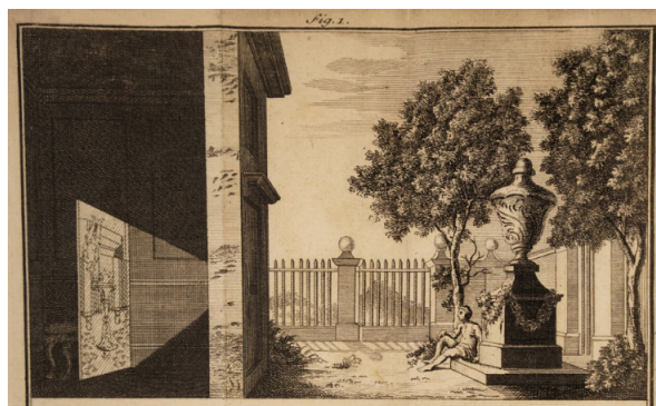
Figure 1: The camera obscura principle, also known as the pinhole camera. The visual scene is projected in a reversed and inverted manner on the wall opposing the hole. Illustration from James Ayscough's A short account of the eye and nature of vision (1755, 4 th edition, public domain)
