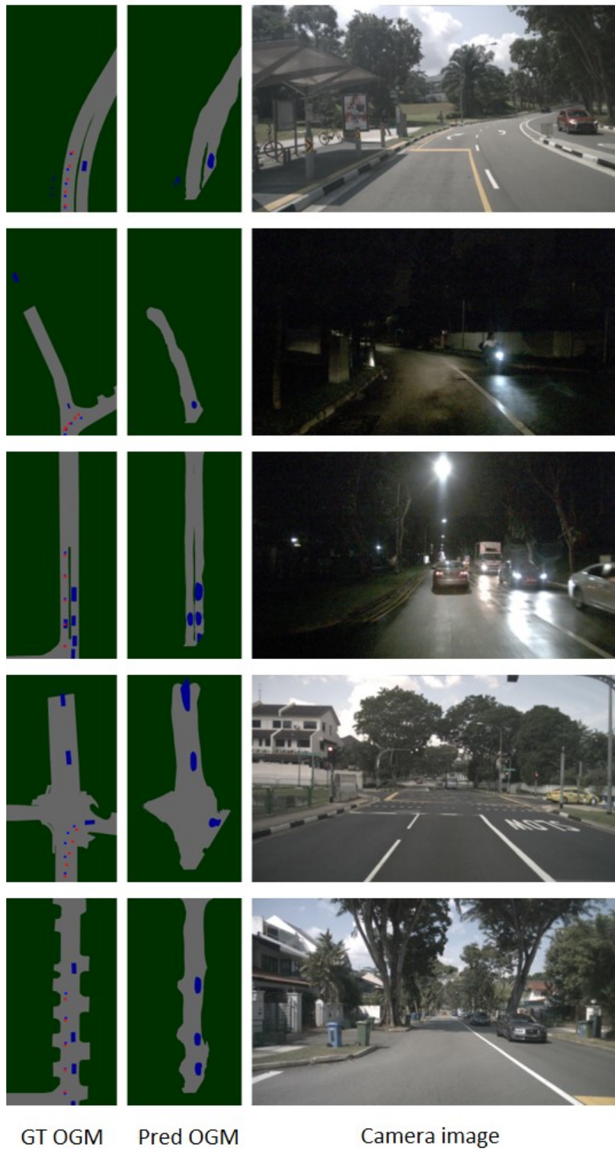
FIGURE 6.3: Qualitative results of our holistic trajectory planning network on nuScenes; blue dots are for ground truth, red dots for prediction.
