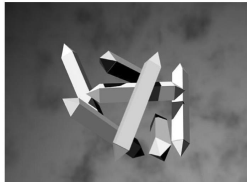
Figure I-30: Schematic view of wax crystallization in (1) Needle-like structure and (2) 3D gel network of needle-like structures 10
