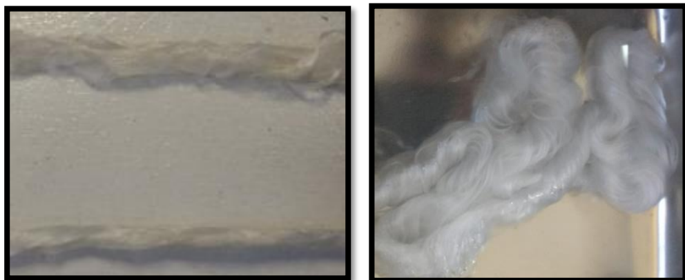
Figure 4-5. Non-coated yarn after the ultrasonic bath after drying (a) and in water (b).
