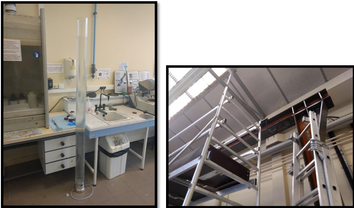
Figure 7-11. Watertightness test of the tube (a) and installing the top bracket (b).
