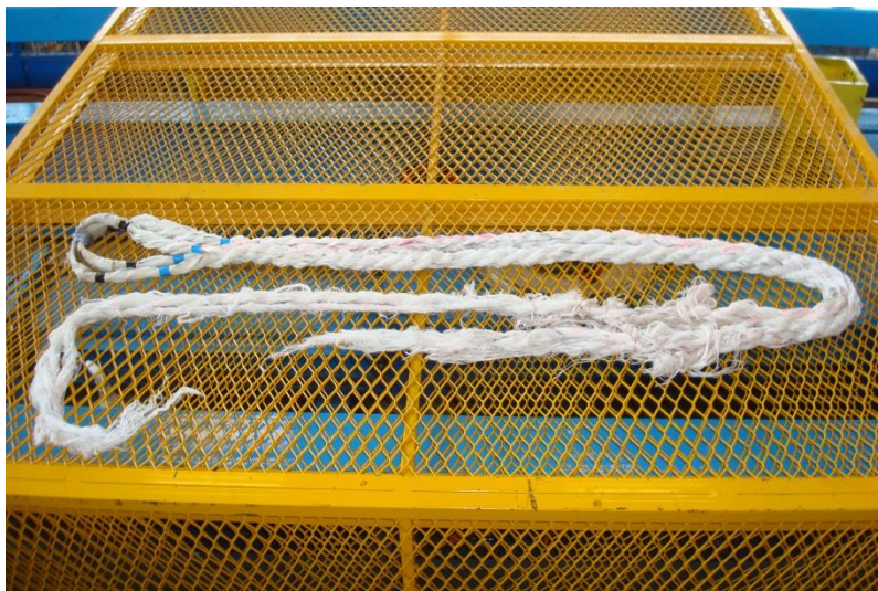
Figure 4-19. Failed 8-tons sub-rope sample after test, showing two broken parts superposed.
