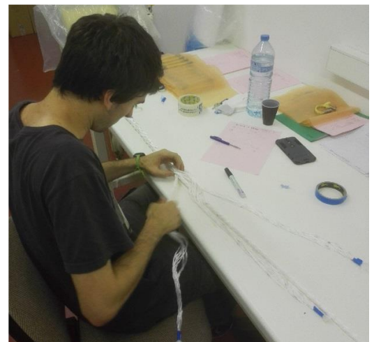
Figure 2-7. Splicing of a 4 ton sub-rop diameter.
