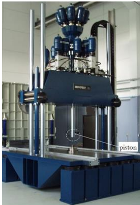
Figure 2-9. Servotest machine used for testing the 4-ton sub-ropes in the mechanical laboratory of ENSTA Bretagne.
