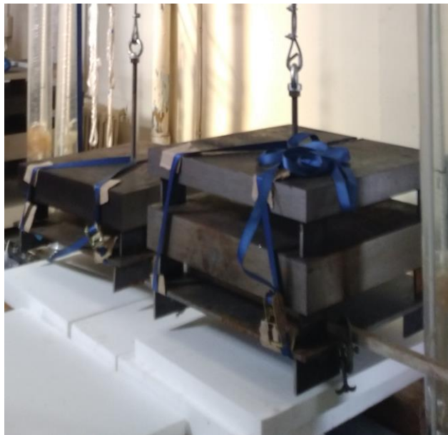
Figure 7-8. Weight of the long-term creep machine.
