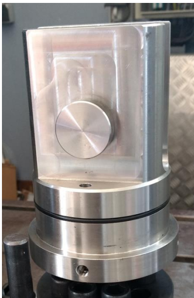
Figure 2-10. Bottom jaw of the experimental setup (left), watering system at the top of the sample (middle) and installed sub-rope (right).
