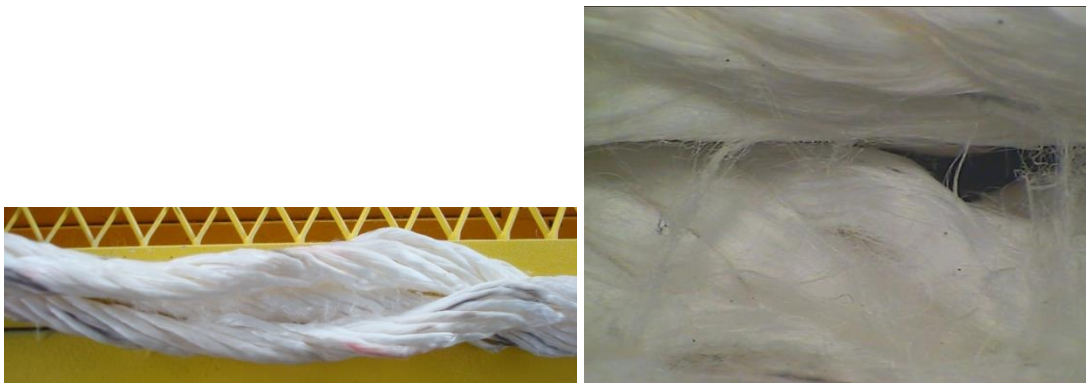
Figure 4-29. Example of internal abrasion in rope sample.
