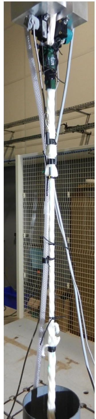
Figure 2-10. Bottom jaw of the experimental setup (left), watering system at the top of the sample (middle) and installed sub-rope (right).
