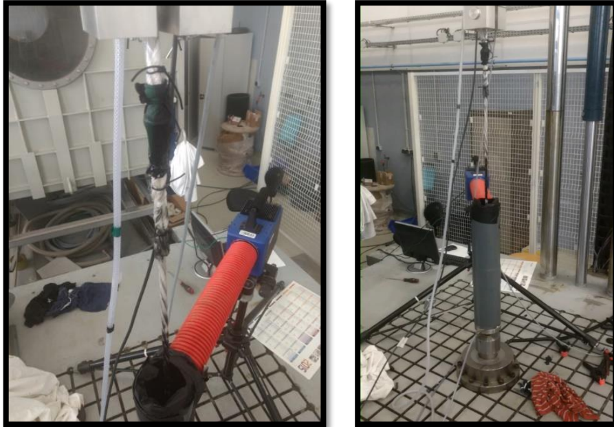
Figure 4-7. 4-tons sub-rope during a fatigue test.
